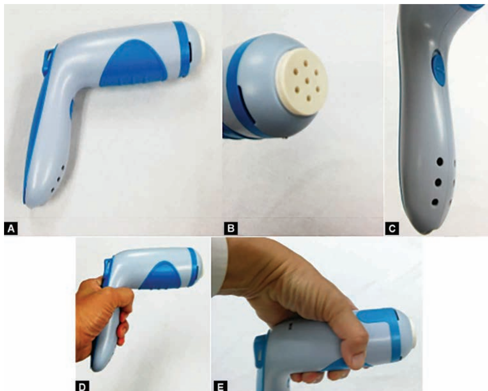
Figs 1A to E: Details on the Energy Accumulator (A) outlook; (B) Ceramic plate with temperature sensors at the hot air outlet; (C) handle with on/off switch and air inlets; (D and E) The 2-way holding of the device
